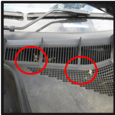
Look for insects, plant material and spiders in and around bonnet grilles.
