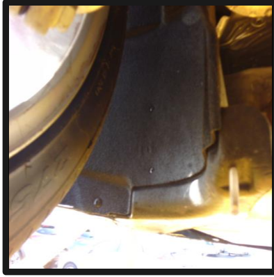
Thoroughly check mudguards, tyres and wheel arches for soil and seeds. Water blasting may be best to remove soil in these areas.
