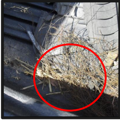
Look for plant material in exterior compartments and trays. Remove any pooled water from the vehicle.
