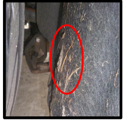
If mud guards are covered in felt, thorough scrubbing or water blasting is often required, especially around the wheel arch.
